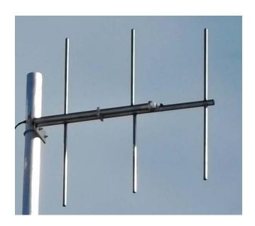
The FMC series of antennas are rugged 3 element Yagi's. They form a single polarization cardioid pattern and have a gain of 4.5 dB. The front to back ratio is between 12 and 14 dB depending on frequency. They can be mounted horizontally or vertically. The FMC is a 50 Ohm antenna.
